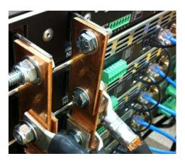
(Figure: 4 Back Panel Parallel Connections)
